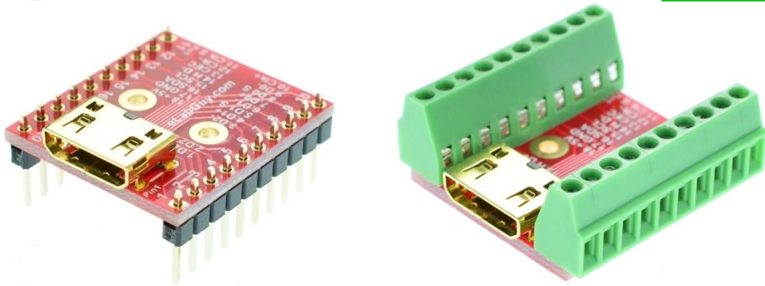
Figure 3: HDMI-CF-BO-V1A various connections
